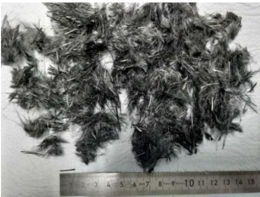
Fig. 8. Matted texture of fibers.
