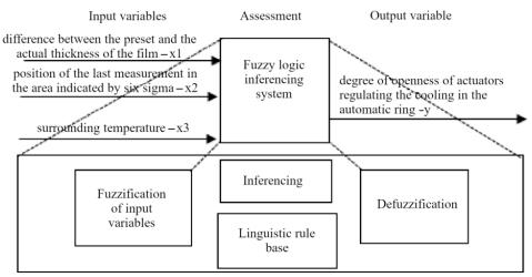
Fig. 4. Inferencing process based on fuzzy logic.
