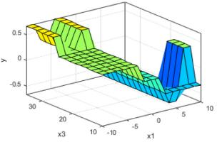
Fig. 6. Graphical presentation of transfer function in the fuzzy controller.
