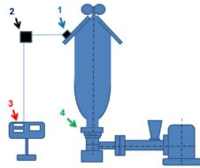
Fig. 1. The concept of application of Fuzzy Logic controller for automatic control of film thickness in the process of extrusion: 1 – film thickness sensor, 2 – measurand converter, 3 – control panel with Fuzzy Logic controller for film thickness adjustment, 4 – segmented cooling ring with automatic airflow regulation.
