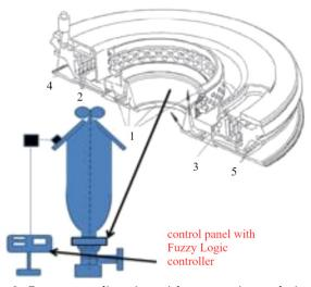
Fig. 3. Segment cooling ring with automatic regulation of film-cooling airflow: 1 – dual-flow cooling ring, 2 – adjusting actuators, 3 – actuator unit, 4 – actuator positioning drive, 5 – perimetric air inlet; arrows mark the outflow of air.
