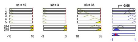
Fig. 7. Fuzzy controller operation example – the degree of opening of the actuators regulating the cooling.
